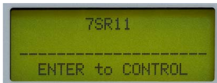
Figure 1-18 Close up of Relay Identifier
