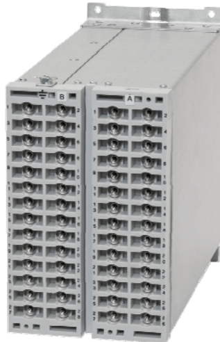
Figure 1-12 7SR11 Rear view of 7SR11 Relay
